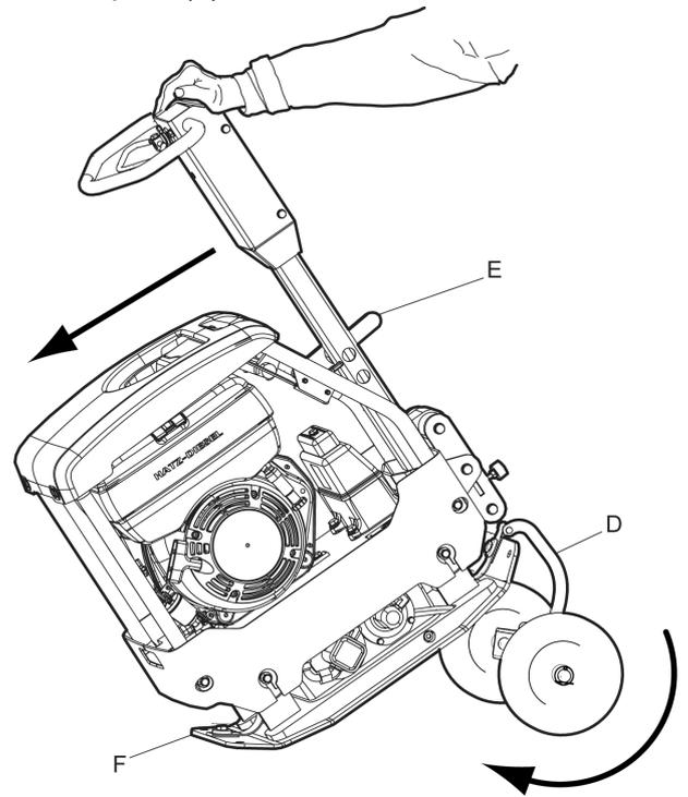
5. Unlock the handle (E) and tilt the machine backwards.
