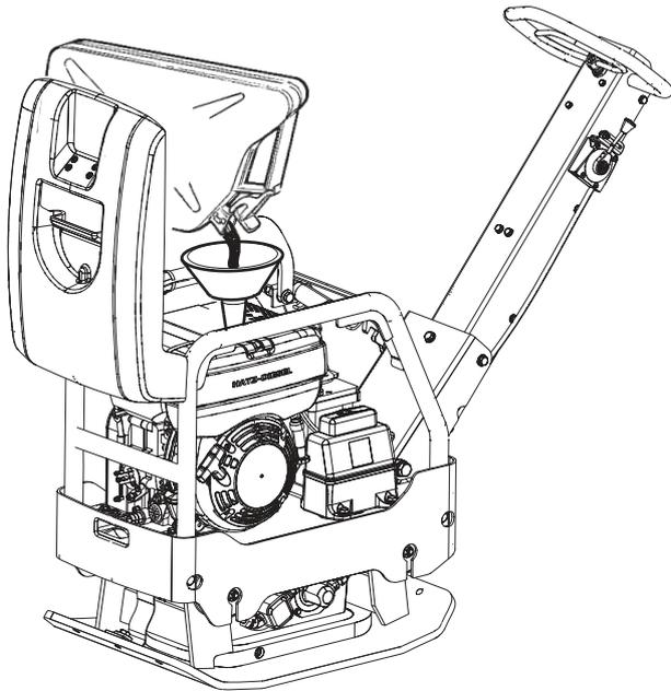
4. Never overfill the tank. Due to the movement of the fuel within the tank, it is possible to have fuel at a higher level than the tank cap, which can lead to a spillage of fuel if the tank cap is opened. This can be avoided by only opening the tank cap when the machine is on level ground and the tank cap is at the fuel tank's highest point.
