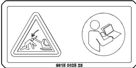
The handle must be locked when in the raised position. Read the instruction manual.
