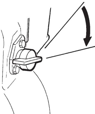
4. Pull out the starter rope until it resists. Release the handle so the starter rope goes back again, and then pull the starter rope until the engine starts.
