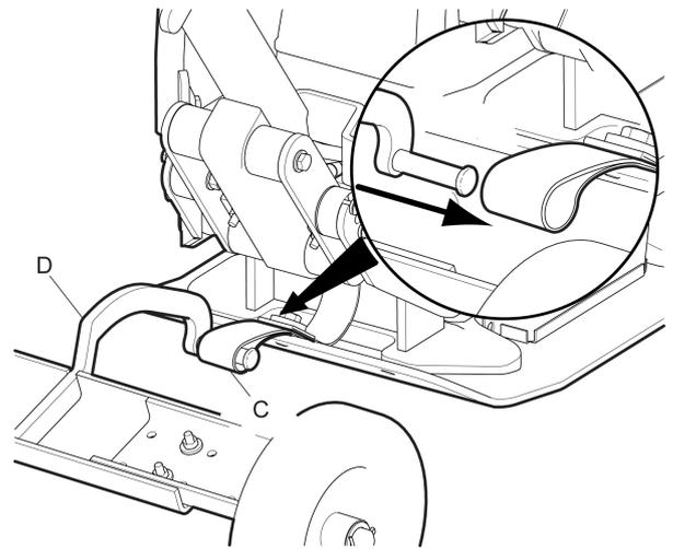
4. Lock the handle (E) and tilt the machine forwards. Fold the trolley (D) in under the bottom plate (F).
