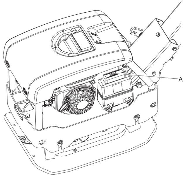
2. Fill up with hydraulic oil if necessary, see chapter "Hydraulic system, changing the hydraulic oil".
