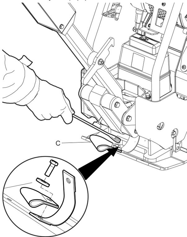
3. Mount the trolley (D) in the trolley strap (C).
