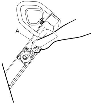
2. Close the choke valve if the engine is cold. If the engine is warm or the ambient temperature is high, close the choke valve halfway or leave it open.
