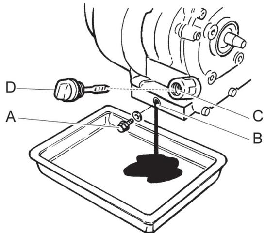
2. Tilt the machine backwards and let the oil drain in a drainage hose.
